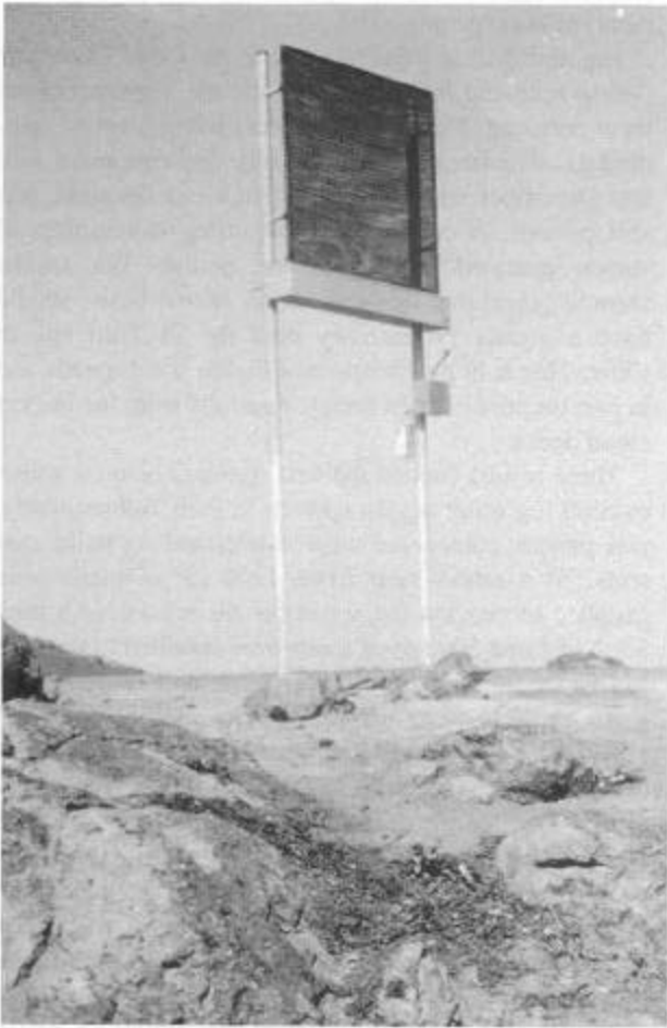
Figure 4. A standard 1 m 2 fog collector used for initial field investigations, Cerro Orara, Peru.
